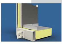
**Inferior thermal break design** with liners moved to exterior of panels.
