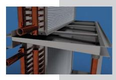
Auxiliary drain pan has potential for water overflow.
