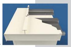
between the roof panel and third-layer roof systemeliminating the possibility of condensation. Outdoor unit roofs are constructed with the same material as the unit exterior liner and panels are broken outwards. No air barrier is provided isolating the unit roof panels and roofing system. Possible point of condensation and water penetration.
