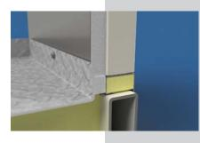
Z-bar is tack welded and caulked – NOT continuously welded. Water leak potential. Z-bar is a thermal bridge.
