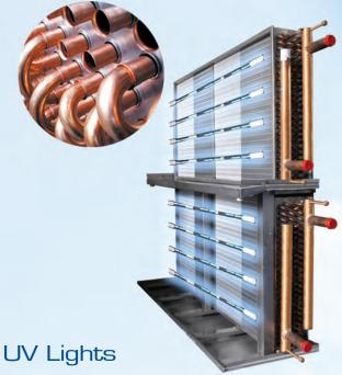
Energy Labs offers flexible and effective high intensity UV disinfection using UV irradiation for air stream as well as surface disinfection. Air stream disinfection, also known as "on the fly kill", is the application of high intensity UVC energy to disinfect a fast moving air stream and neutralize microbes including viruses, bacteria and mold spores.
